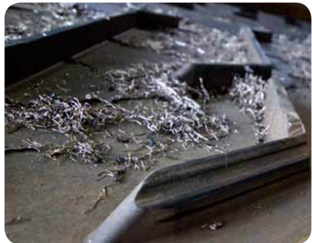
High quality steel deriving from tyre recycling, a material commonly used and requested by e.g steel works.
