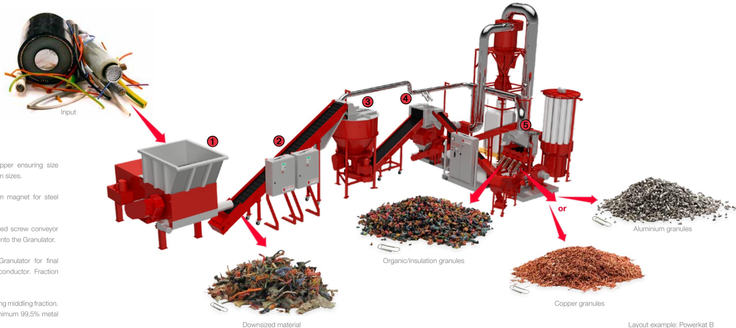
**1. Rough Chopper.** Single shaft pre-chopper ensuring size reduction down to approx. 10-25 mm in fraction sizes.
