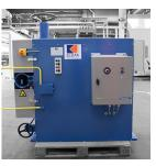
The Cable Strippers peel cables with a diameter from 10-150 mm. Capacity up to 30 meter/minute.
