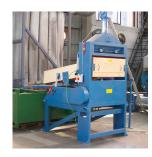
**The Classifier** is perfect for recovery of metals remaining in the plastic fraction. Reduction of metal losses down to 2,0 %.
