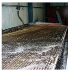
**The Water Separation Table** recovers metals remaining in the plastic fraction. Reduces metal losses down to as little as 0,2 %.
