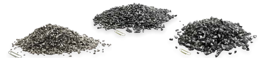
Granules - various sizes after Fine Granulator and Separation Table
